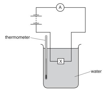
When the temperature of the water is increased, the reading on the ammeter increases.
